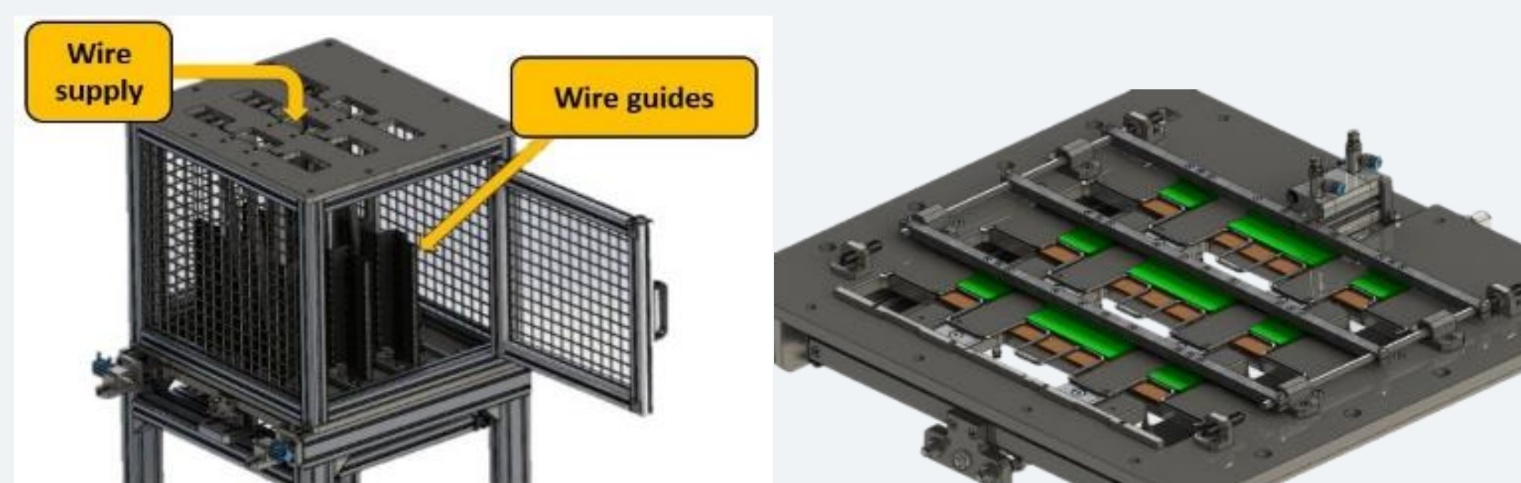
Fig. 3. - Guide columns and the supply system of the wires to the jig in the drawer, respectively
