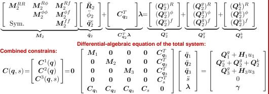
The equation of motion of the mast, which is an elastic body, is formulated using the floating frame of reference formulation. Since the carriage runs on the mast, it becomes a problem of moving boundary conditions. Therefore, a dummy variable *s* is introduced to express the connection of both bodies. Using differential algebraic equation, dynamic model that considers the coupling of motion and vibration is obtain.
