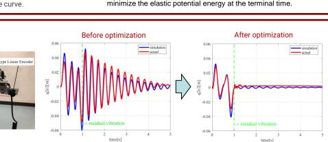
In order to confirm the effectiveness of the proposed method, we built an experimental device for a stacker crane. These figures show the lateral deformation of the mast, where the blue line is the numerical simulation result and the red line is the experimental result. It can be confirmed that the numerical simulation and experimental results are in good agreement. It can also be confirmed that residual vibrations can be significantly suppressed by applying the proposed method.
