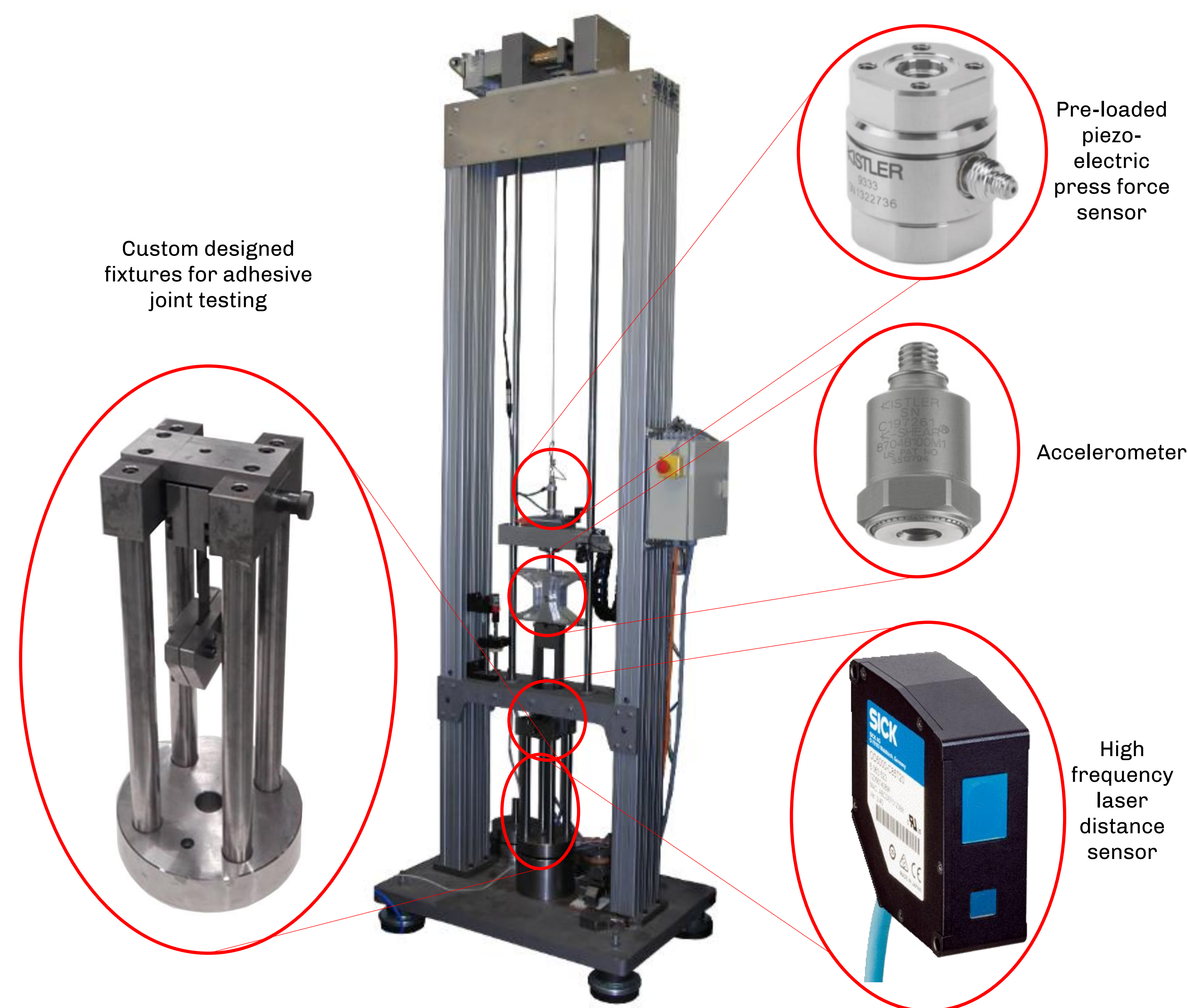
Figure 1 – Drop weight machine, primary sensors and custom fixture.
