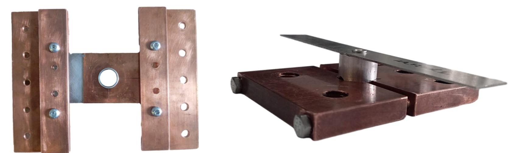
Figure 4– Joints mounted in the experimental fixtures: (left) hole-hemmed joint, (right) tube-fit joint.
